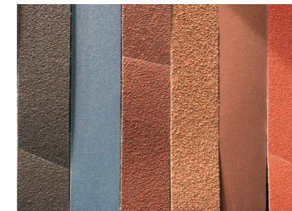
紙(基材)に研磨材をくっつける研磨材用樹脂 Resin which bonds grinding compounds to a paper substrate
